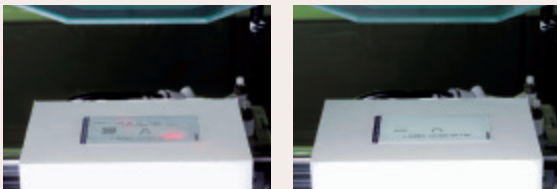
System that uses laser beams to rewrite or delete information in just a few seconds
